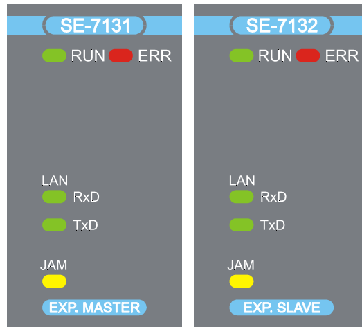
Fig.2.21 Detail of indication of system expanders
